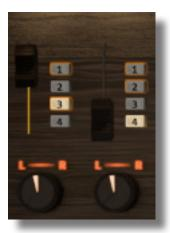
Select one of the 4 IR Sends and adjust the volume slider. If an AUX Send is active the corresponding button will lit up.
